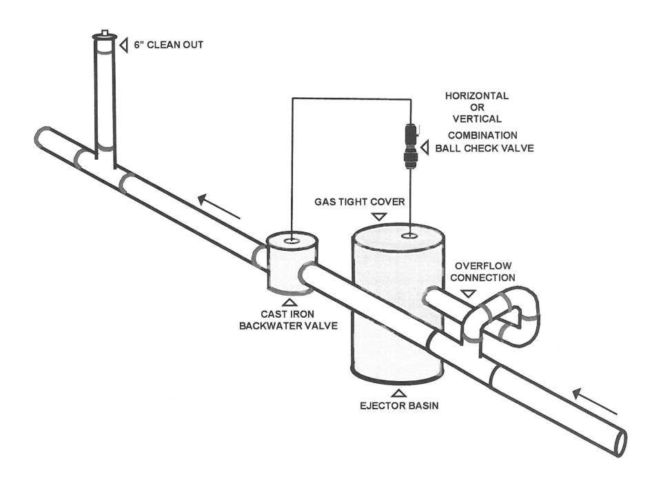
Overhead Sewer Ejector Discharge Disconnect Existing Soil Stack & Reroute To Underground Connection
